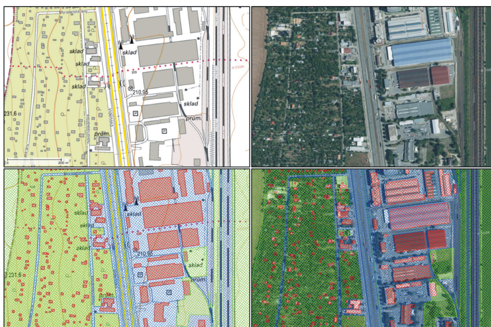
Fig. 3: Categories of building surface, impervious surface, and pervious surface after the reclassification of ZABAGED (left) and its checking against the background of an aerial image (right) Source: authors' elaboration (basic data: ZABAGED and Orthophotomap are provided by ČÚZK, 2015)
