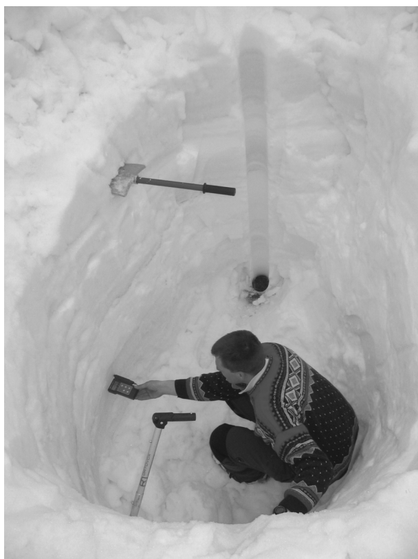
Figure 2 Measuring of temperature in snow cover after a sample was taken with a tube. Photo: M. Ogrin.
